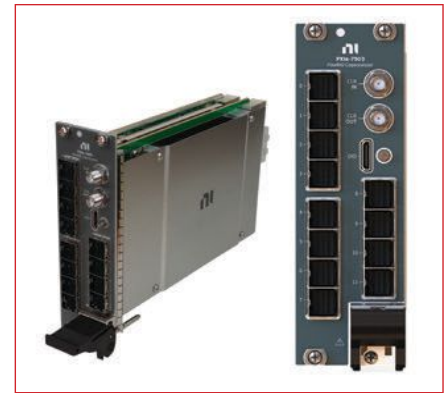
▲ Fig. 8 NI PXIe-7903 Flex-RIO HSS module. Source: Based on Xilinx Virtex UltraScale+ VU11P FPGA with 48 multi-gigabit transceivers.
